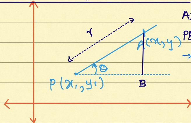
$$\begin{aligned} AB &= y - y_1 = r \sin \theta \\ PB &= x - x_1 = r \cos \theta \\ \Rightarrow \frac{x - x_1}{\cos \theta} &= \frac{y - y_1}{\sin \theta} = r \end{aligned}$$
